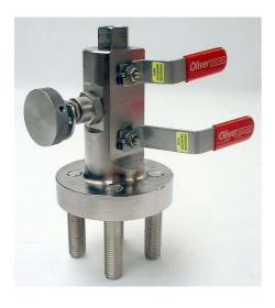
Machined from a single piece of 'grain flow controlled' forging, this valve features two inline ball pattern primary and secondary isolating valves and a heavy duty ball vent valve.
