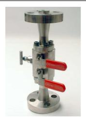
Machined from a barstock forging, this valve features two inline ball pattern primary and secondary isolating valves and a heavy duty needle vent valve.
