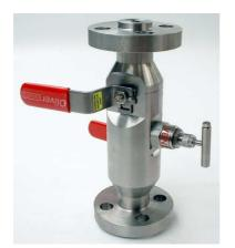
Machined from a single piece of 'grain flow controlled' forging, this valve features two inline ball pattern primary and secondary isolating valves and a heavy duty needle vent valve.
